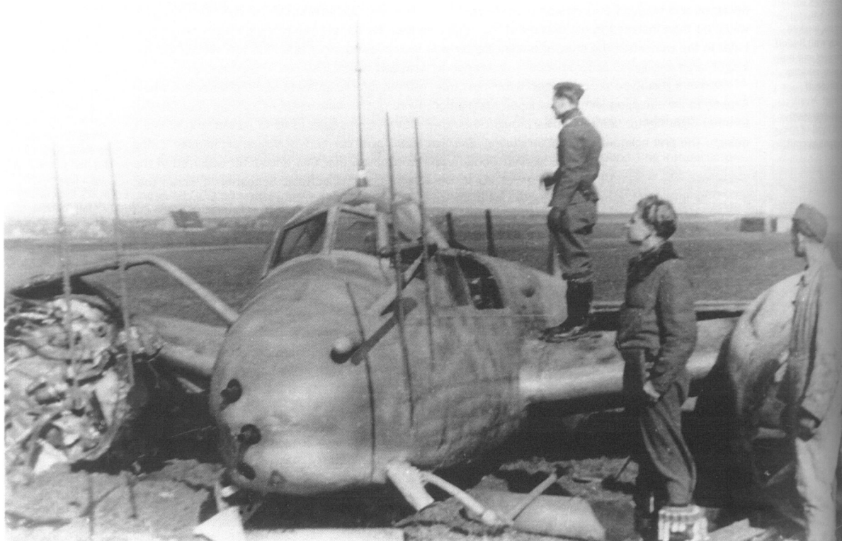
THIS PAGE: A crash-landed Ju 88 C-6 clearly showing the 'Schräge Musik' installation of two MG151/20 cannon protruding from the fuselage. This particular aircraft, R4 + LS, W.Nr. 750811, was being flown on a daylight mission on 30 January 1944 by Hptm. Friedrich Tober of III./NJG 2 when it was attacked and shot down by a P-47. Tober's machine crashed in a field south-west of Hardenberg, as a result of which it was written off.
