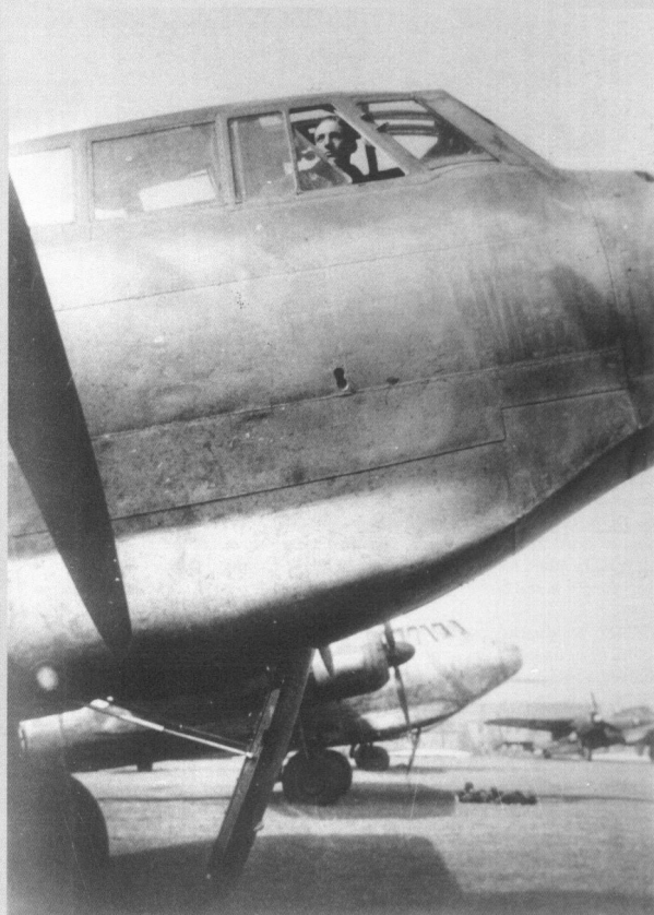
ABOVE AND BELOW: Two further examples of the continued use of darker night fighter colours may be seen on these Do 217s where the upper surfaces and fuselage sides have been darkened, one with mottling ( BELOW ) and the other with a solid application of a single colour, presumably 75.
